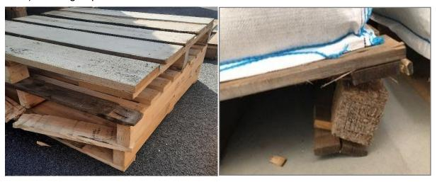
c) Minimum load capacity broken
